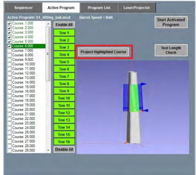
Figure 8. Electroimpact Part Program Display
