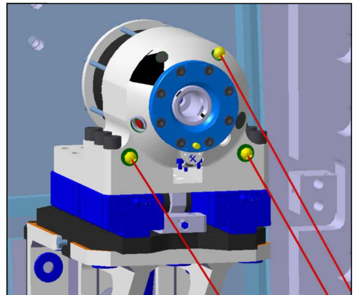
*Figure 3. Ball Clamp Interface*
