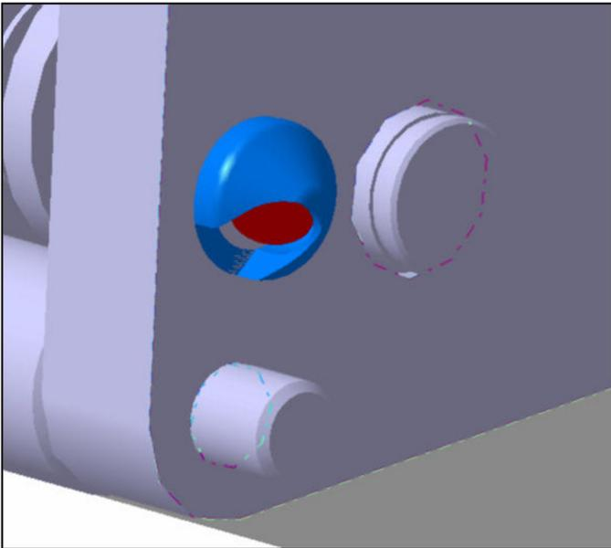
Figure 4. Laser Tracker Target Cover Concept
