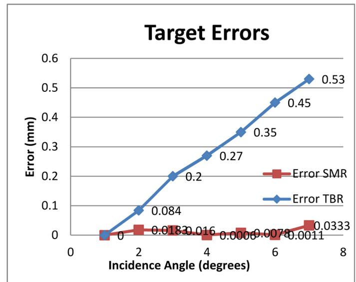
Figure 5. SMR vs Solid Prism
