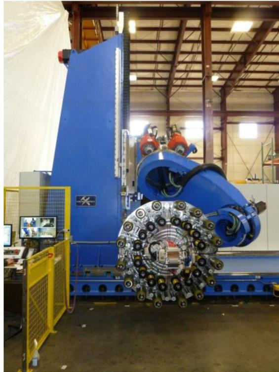
**Figure 9. Electroimpact AFP machine with new rotary kinematics.**
