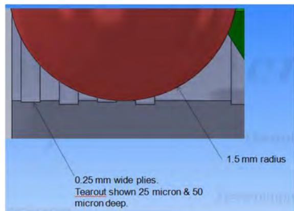
Figure 6. Hole probe diameter size effects.
