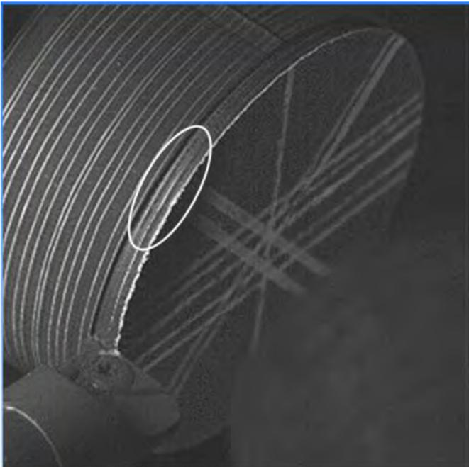
*Figure 9. Cutting action investigated by turning CFRP on lathe.*
