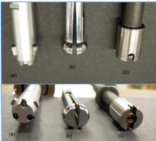
Figure 5. Hole probe types for 11.11 mm. (a) 3-point (b) split ball (c) 2-point ball plug.
