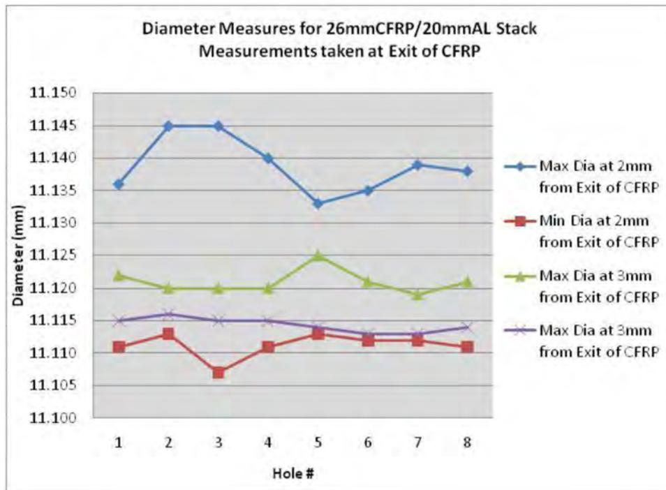
Figure 8. Axial location affects diameter measurements.
