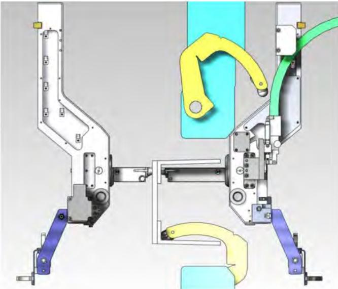
**Figure 4. Fastening heads interacting with the spar components.**
