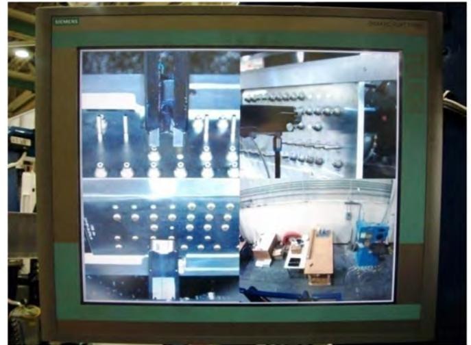
Figure 9. The four camera digital display used on the new ASAT2 system.
