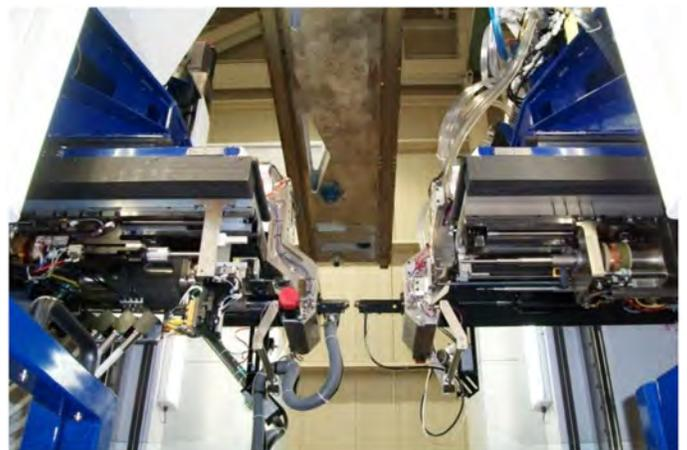
*Figure 3. Fastening heads of the ASAT2 machine.*
