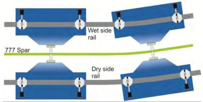
**Figure 5. Dry and wet carriage transition through the spar inflection.**
