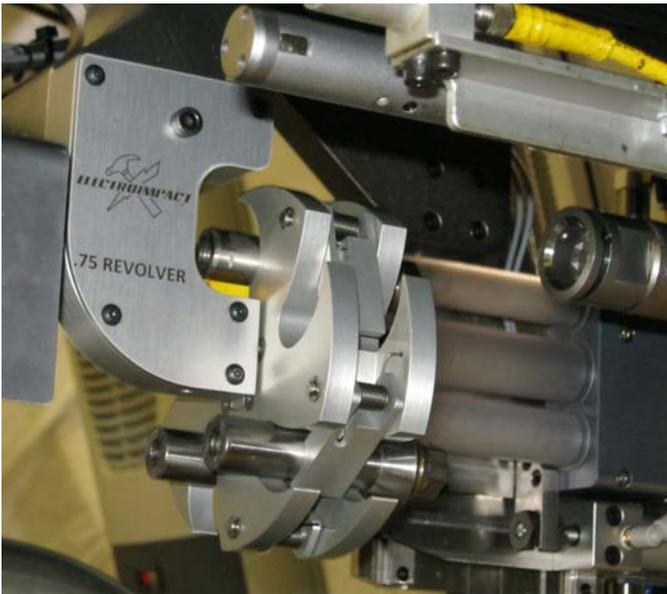
*Figure 8-Revolver Feed Cartridge*
