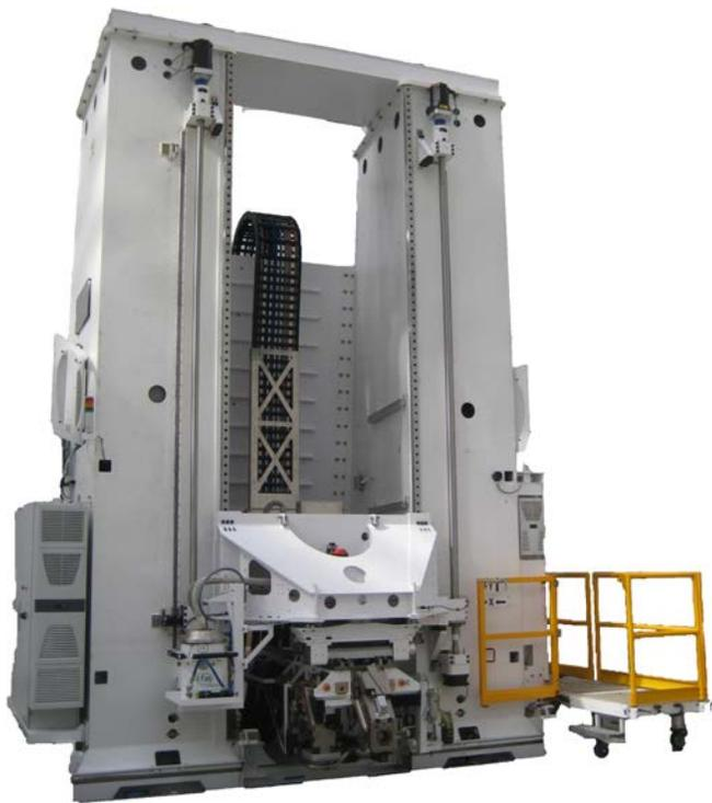
*Figure 1-Lean Technology Drilling Machine (LTD)*
