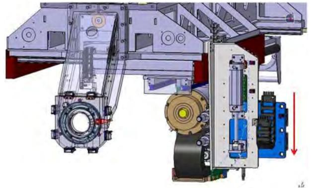
**Figure 9. ATS selector plate shuttles to alternate position.**
