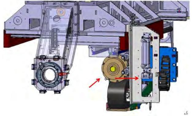
**Figure 8. First gripper retracts to clear spindle.**
