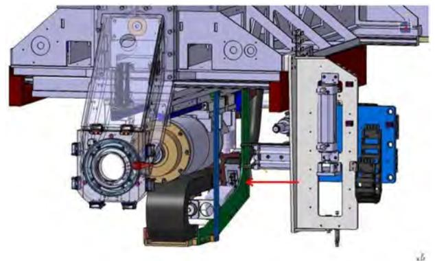
*Figure 5. First gripper extends to receive tool from spindle.*
