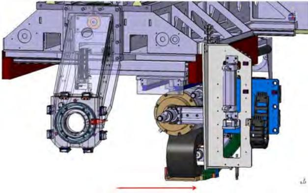
**Figure 6. Shuttle movement loads cutter into Position 2 gripper.**
