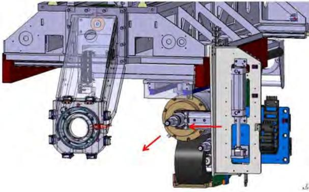
*Figure 10. Second gripper extends to place new tool in spindle.*
