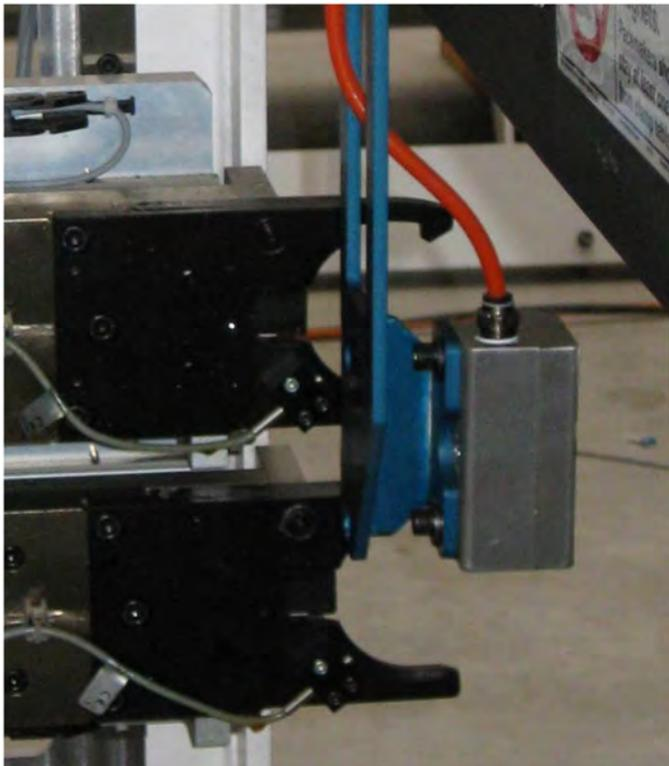
**Figure 7. Taper blast clears debris from tool holders.**
