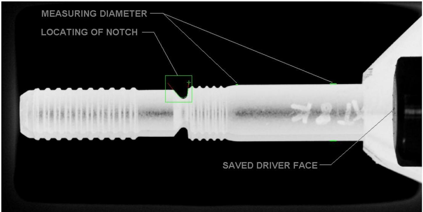
Figure 3: Measurement of Bolt
