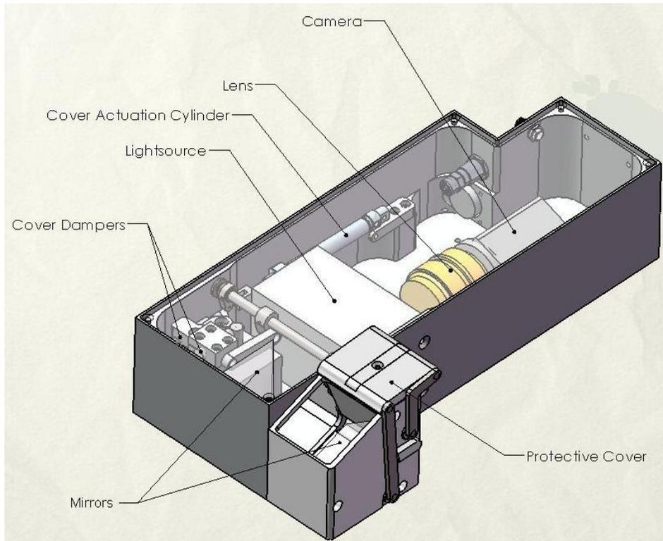
Figure 1: Bolt Camera Assembly
