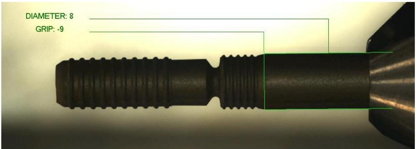
Figure 2: Operator Display of Measured Bolt Dimensions
