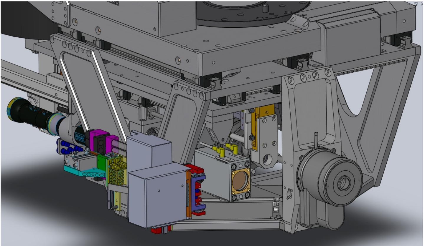
Figure 1: Aircraft Fastening/Drilling Machine End Effector
