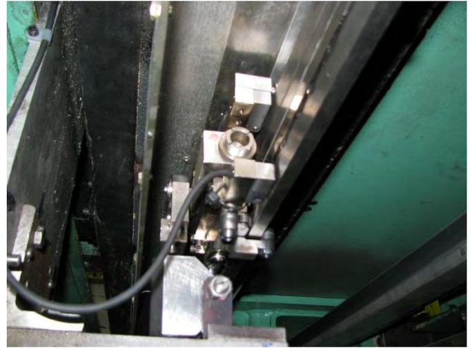
Figure 2: Installation of LM10 linear scale
