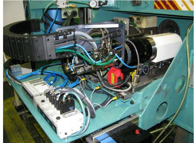
Figure 5 Precise drill spindle mounted on the new dry side shuttle table
