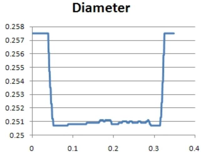
**Figure 8.** [2] Hole profile results using automated probe
