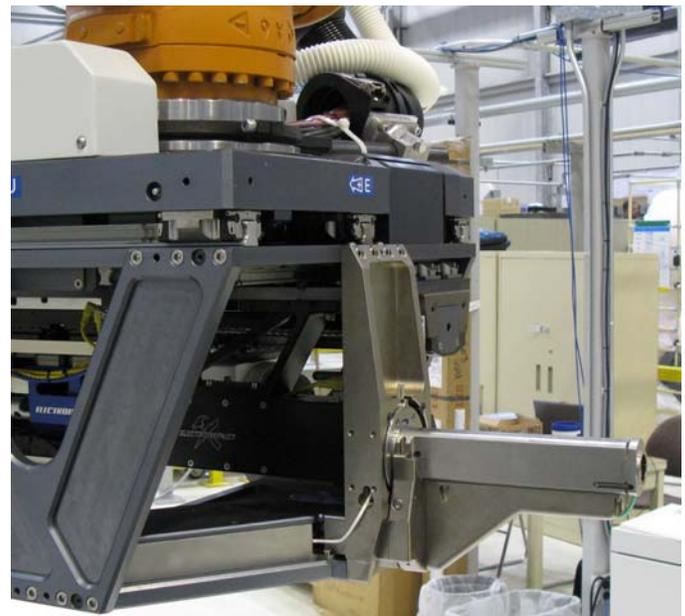
**Figure 4.** Special long nose with compliant tip, flood coolant delivery, and vacuum extraction
