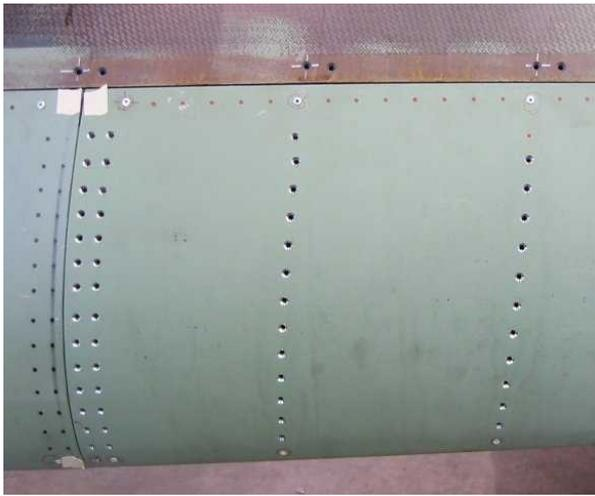
**Figure 5.** [1] High-curvature leading edge showing tack fasteners and drilled hole patterns
