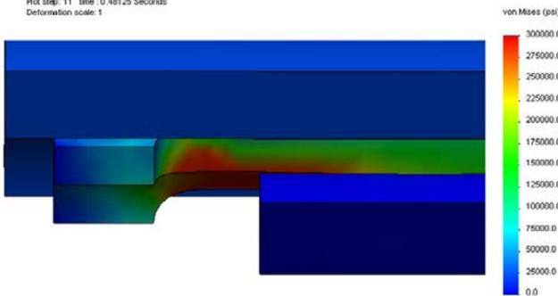
Figure 32. Maximum stresses during clamping.
