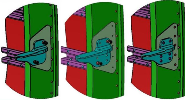
Figure 9 – Sequence of determinant clamp with SSSF, drill, and final fastening
