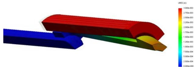
Figure 35. Residual deformation after Case 2A loading
