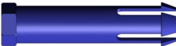
Figure 17. Machined collet body.
