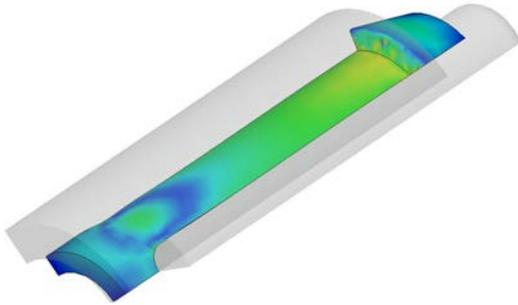
Figure 31. Maximum stresses during clamping – top view.
