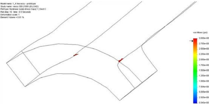
Figure 28. Volume of material that has exceeded yield levels.
