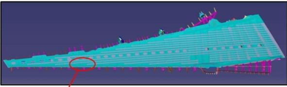
Compare the relatively few SSSF needed to adequately clamp and dowel this wing box together to the more traditional wing build wherein nearly every hole needs a dowel pin or a Cleco-type fastener; please see Figures 15 and 16.
