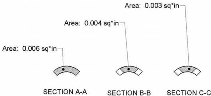
Figure 21. A single finger for a typical Ø 1/4 inch SSSF is shown in the post heat treat condition; multiple section planes are shown.
