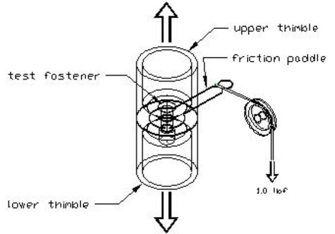
Figure 42. Tension testing per MIL-STD-1312-16
