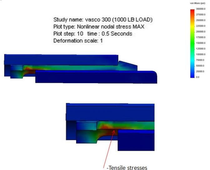
Figure 26. Maximum stresses during clamping.
