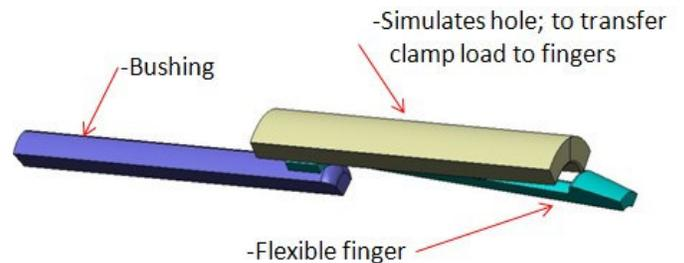
Figure 19. Sectioned flexible finger, bushing, and hole models
