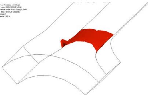
Figure 33. Volume of material that has exceeded yield levels during maximum clamping.
