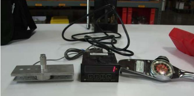
Figure 36. Test setup. Load cell with digital readout, SSSF ( $\varnothing$  1/4 inch), torque wrench. This is shown at the start of testing – fingers are only opened to trap the stack of 2 plates and the load cell.
