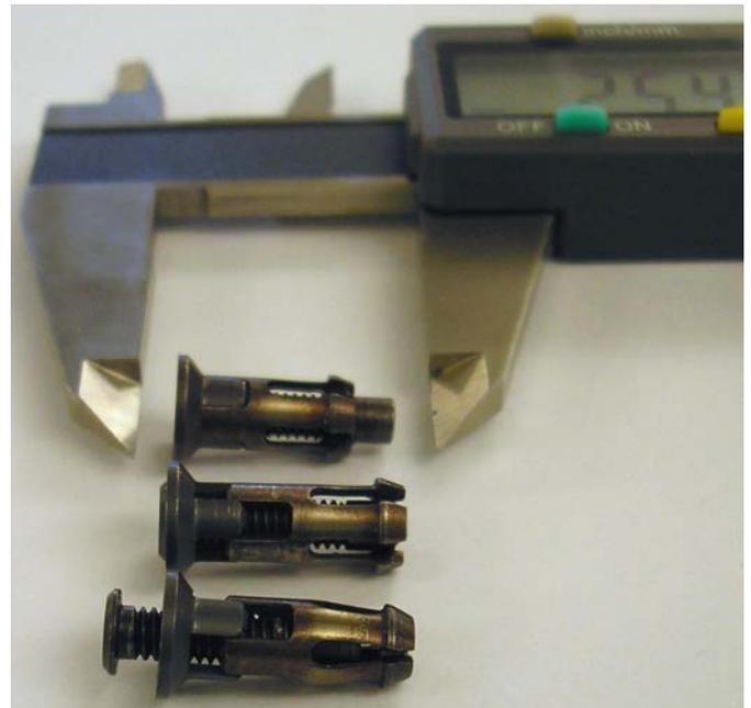
Figure 4. Photograph of Ø1/4 flush head SSSF design – side view
