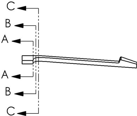
Figure 20. A single finger shown in the post heat treat condition depicted with multiple section planes.
