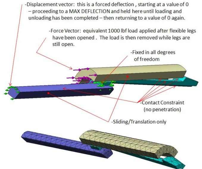
Figure 25. Model and meshing for Case 2 loading
