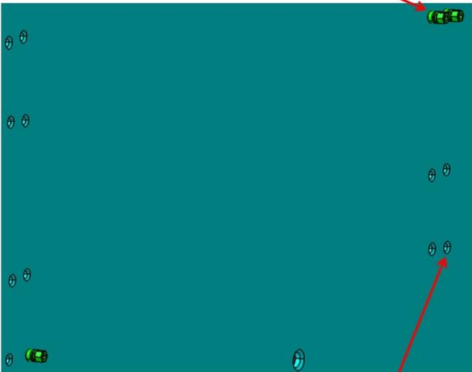
Typical  $\text{Ø}5/16$  inch nominal, drilled and countersunk hole, through cover and rib foot. Installed near to “doweling”, high clamp force SSSF.
