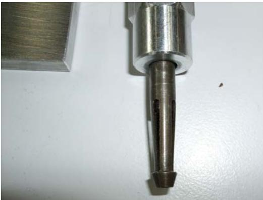
Figure 38. The tool is reverse torqued until it returns to its neutral state. Notice that the fingers are touching at the tips. This suggests that no noticeable residual
