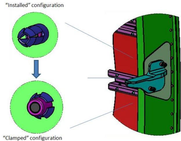
Figure 8 – Tail configuration of SSSF in a determinant assembly
