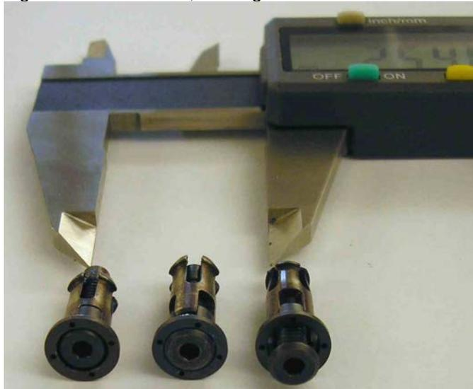
Figure 41 Three, Ø1/4 inch, flush head SSSF, isometric view from the head side.
