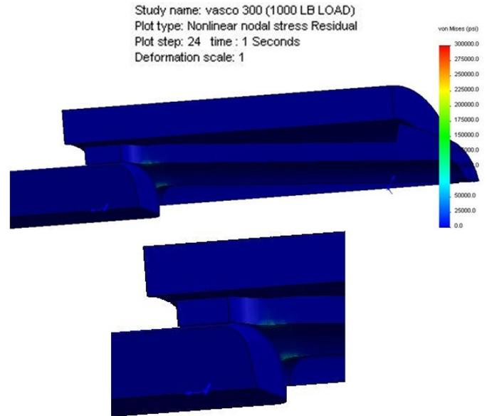
Figure 29. Residual stresses after Case 2 loading
