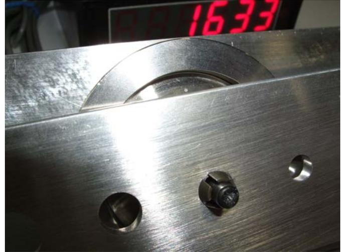
Figure 39. The tool is torqued until the load cell reads approximately 1600 lbs (a little over to account for any error) which corresponds to the Load Case 2A in the FEA section. This test is designed to push the fingers past their design point and compare to the FEA analysis.
