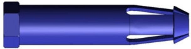
Figure 18. Fingers deformed as after heat treat.
