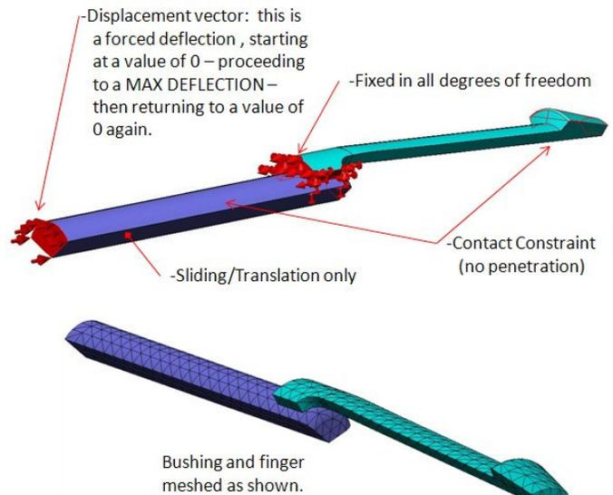
Figure 22. FEA constraints for fingers opening and closing.
