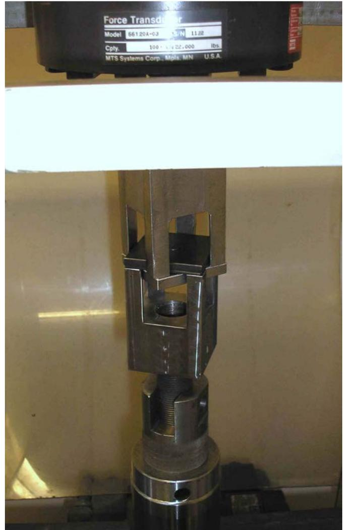
Figure 43. Star coupon testing in tension/compression machine.
