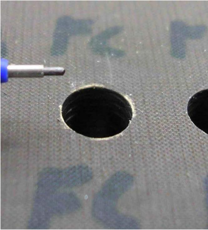
Figure 49. Tail-side hole specimen, after SSSF was installed with 20 in-lb of torque. Note: The pencil diameter shown for reference is 0.7mm (0.028 inch.)
