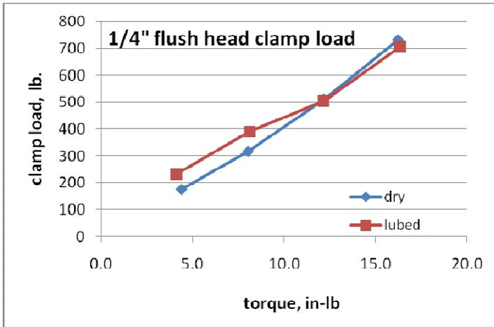
Figure 44. Clamp load versus torque for a Ø1/4, 100° countersunk SSSF.
