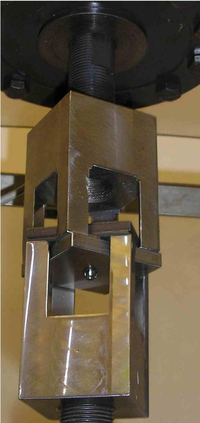
Figure 46. Fatigue test of a SSSF, tail isometric view
