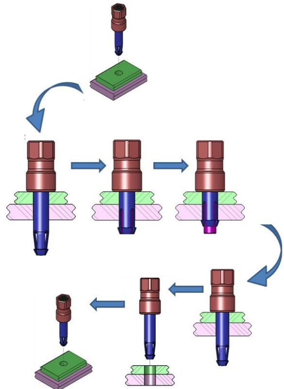
Figure 1. Using a single-sided slave fastener
