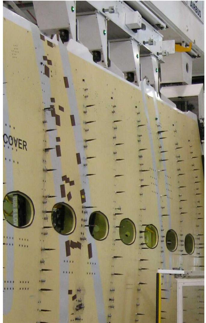
Figure 15 – Traditional outer wing box build using dowel pins and Cleco-type fasteners.
