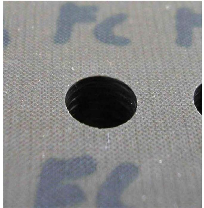
Figure 47. Tail-side hole specimen, before SSSF
