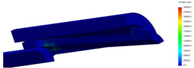
Figure 34. Residual stresses after Case 2A loading
