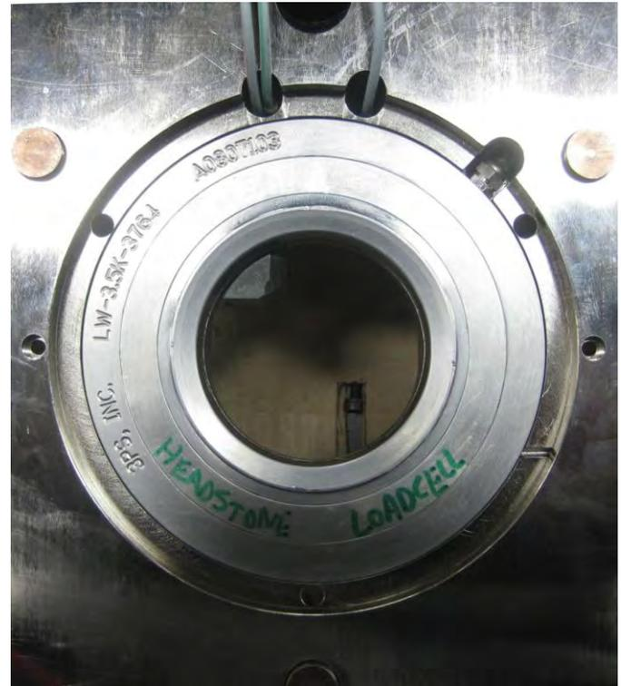
Figure 7 - Doughnut load cell in partially assembled headstone
