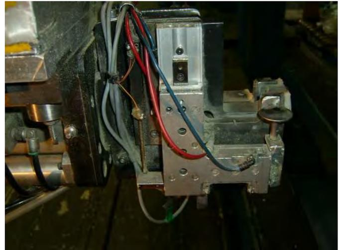
**Figure 4 Tail stone with tracer mechanism**
