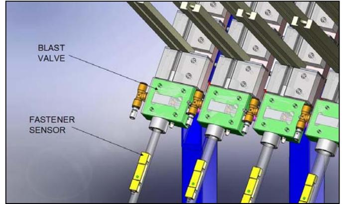
Figure 3. Blast Valves
