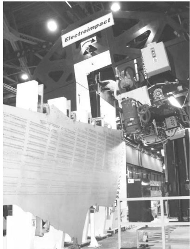
Figure 1. SA2 wing panel fastening machine.
