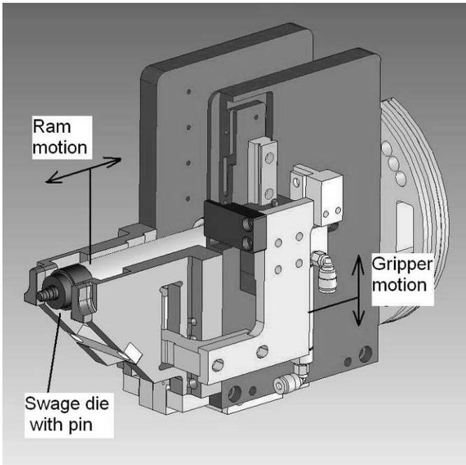
Figure 10a. Anvil for straight collar installation (ram in swaging position).
