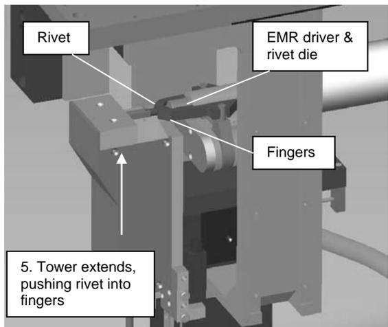
Figure 5b. Rivet is fed into EMR fingers.
