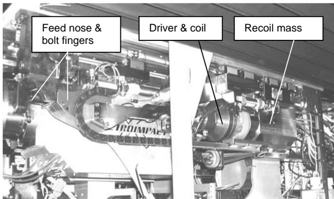
Figure 7. Electromagnetic bolt insertion tool (EMB).
