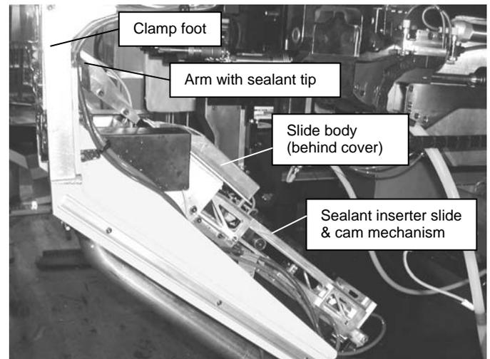
Figure 6. SA2 sealant inserter.
