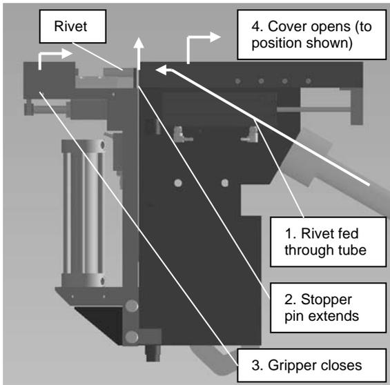
Figure 5a. Rivet feed sequence to injector.
