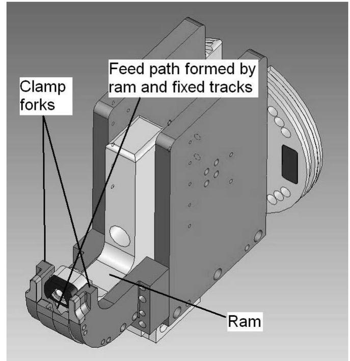
Figure 9. Anvil for offset collar installation.
