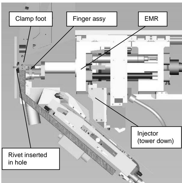
Figure 5c. Fingers insert rivet as EMR moves to panel.
