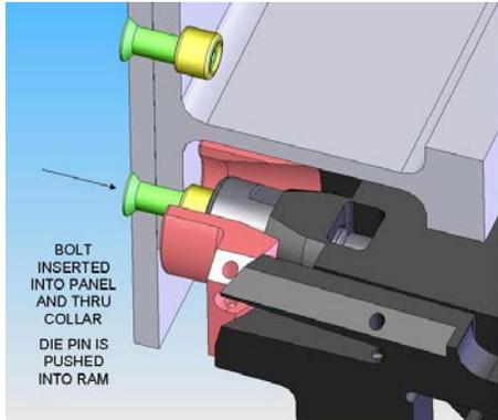
Figure 12: Bolt and collar position check
