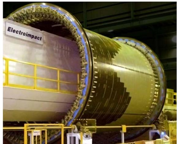
Figure 2: Boeing 787 One-Piece-Barrel (OPB)
