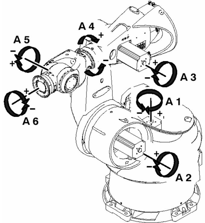
Figure 3. KUKA Robotics KR 360/2 Robot.
