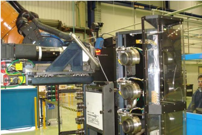
Figure 4. End effector in tool change process.
