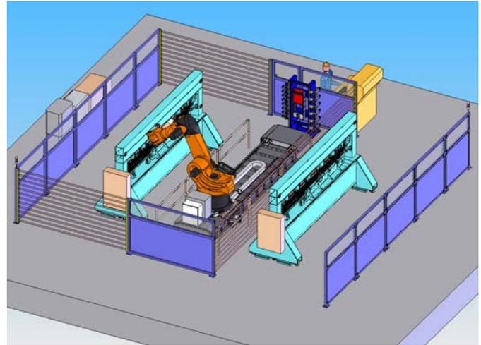
Figure 5. Robot cell layout showing zone 2 active.
