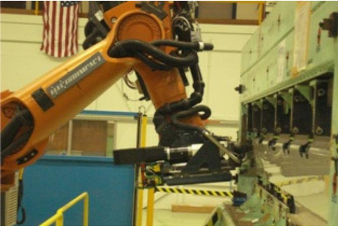
Figure 2. 737 Aileron Robot working with an existing jig.
