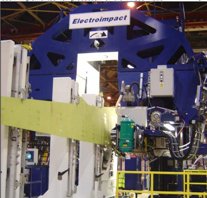
Figure 1: The SA2 machine in the Airbus factory in Broughton, UK Nov. 2006 showing the vertical orientation of the wing skin
