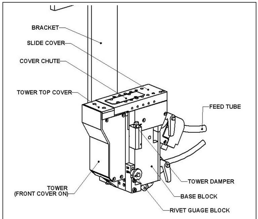
Figure 3: Diagram of the major components comprising the rivet injector
