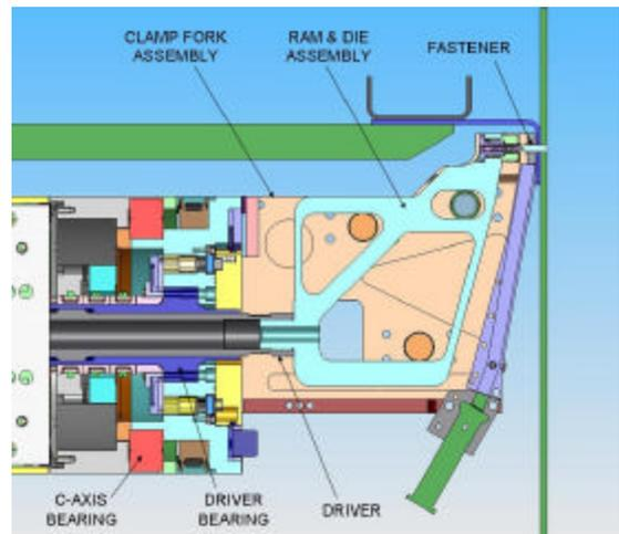
Figure 12: Tooling Layout
