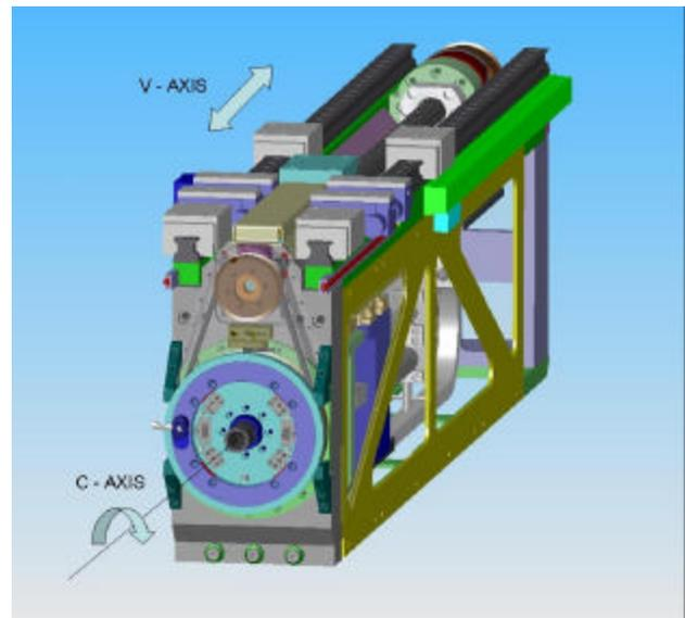
Figure 8: Inner Machine True Offset Head
