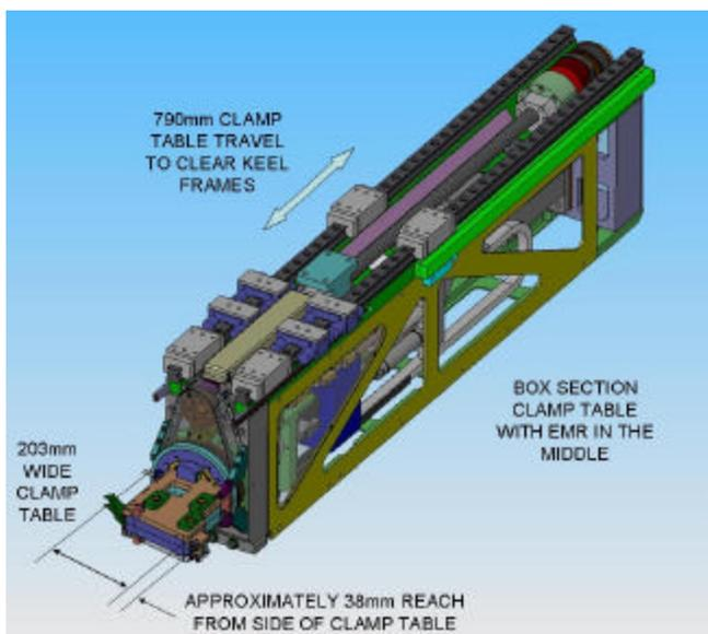
Figure 16: Inner Machine Head
