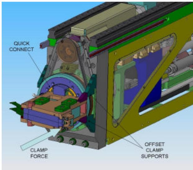
Figure 13: Clamping Loads
