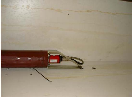
Figure 6, Linear scale buried inside cylinder measures vertical position.
