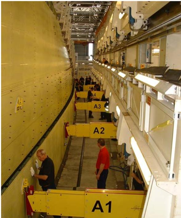
Figure 1, Panel supported by Panel Loaders in wing form prior to engagement with sub-structure.
