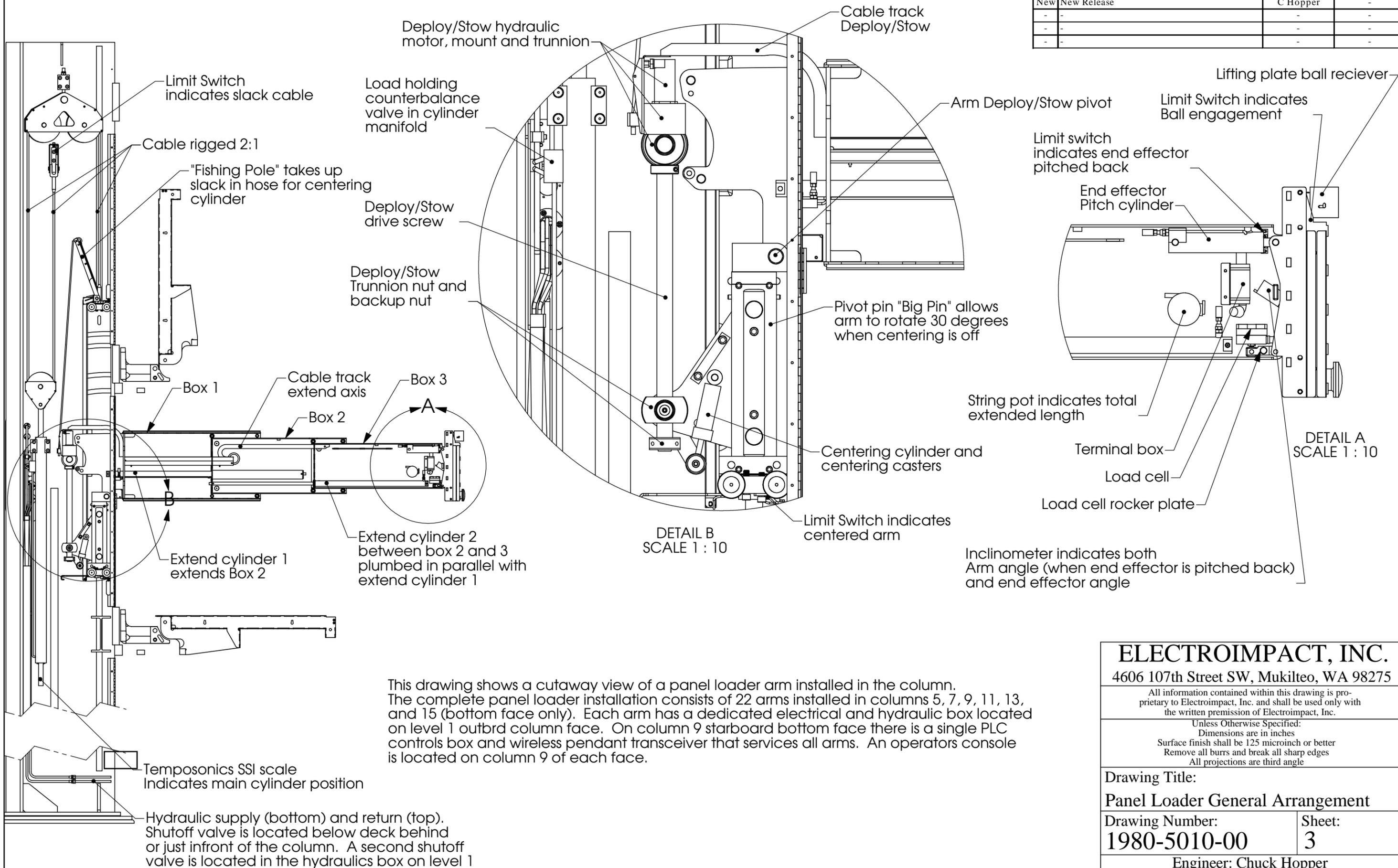
This drawing shows a cutaway view of a panel loader arm installed in the column. The complete panel loader installation consists of 22 arms installed in columns 5, 7, 9, 11, 13, and 15 (bottom face only). Each arm has a dedicated electrical and hydraulic box located on level 1 outboard column face. On column 9 starboard bottom face there is a single PLC controls box and wireless pendant transceiver that services all arms. An operators console is located on column 9 of each face.
