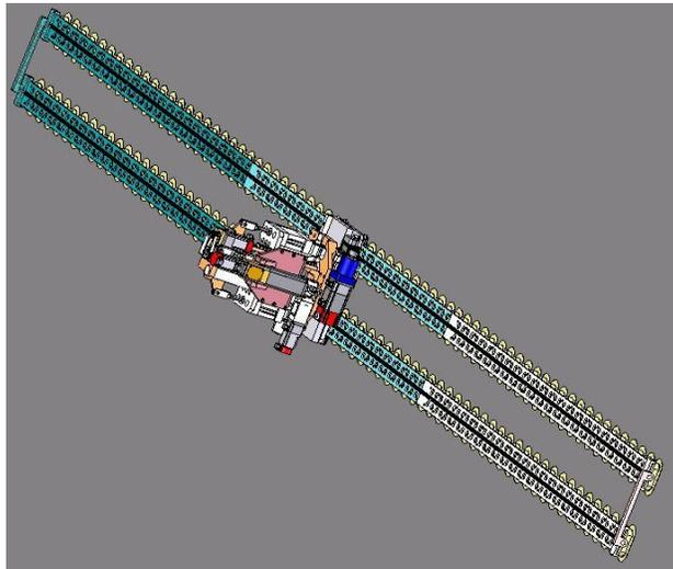
Figure 11: Interlocking Rail Sections
