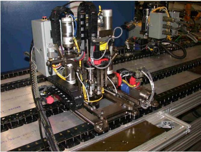
Figure 6: High Torque Flex Track
