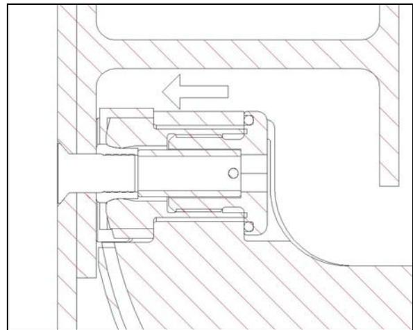
**Figure 11 - Step 7:** Swage collar with EMR
