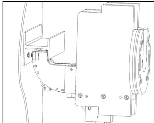
**Figure 12 - Step 8:** Strip die off of collar and unclamp
