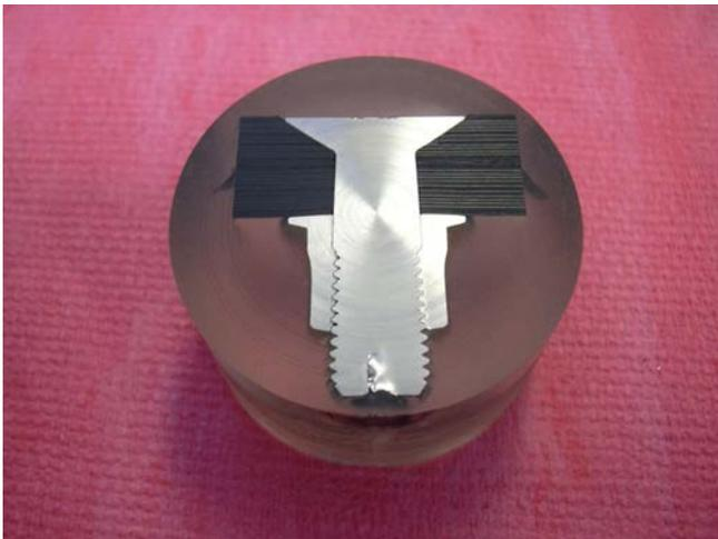
Figure 5 – Sectioned mold
