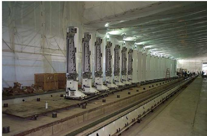
Figure 5: Initial installation of A380 panel-build posts & formboards on-site at Broughton, N. Wales
