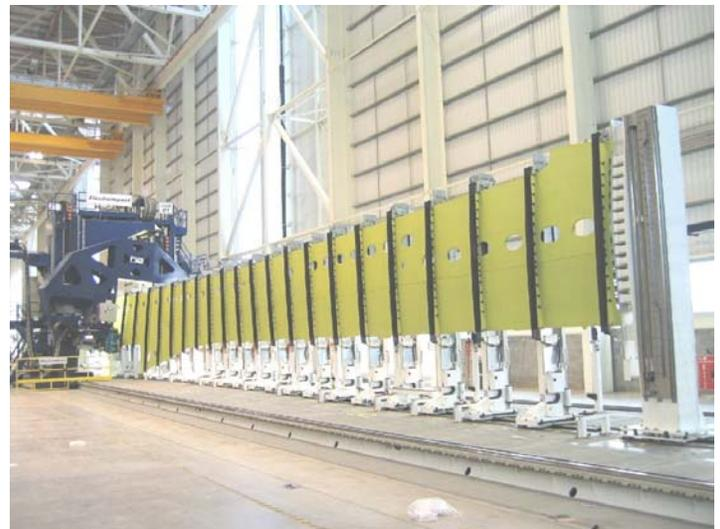
Figure 1 Two tower riveting machine
