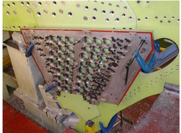
**Figure 1 - Drill jig on A340 gear rib area**
