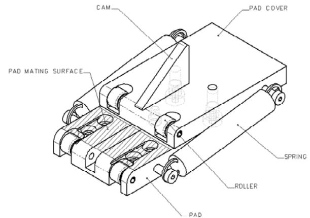
**Figure 10 - Machine Pad**
