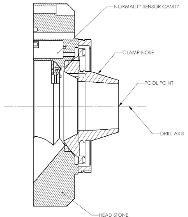
**Figure 5 - Cross section of head stone and clamp nose**
