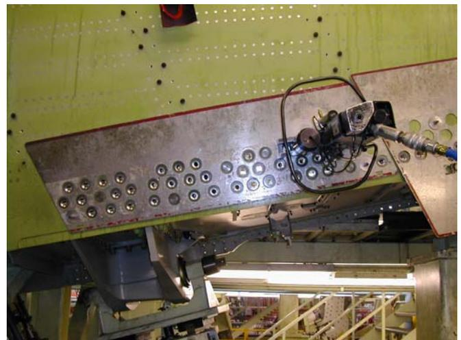
**Figure 2 - Pneumatic drill and template**
