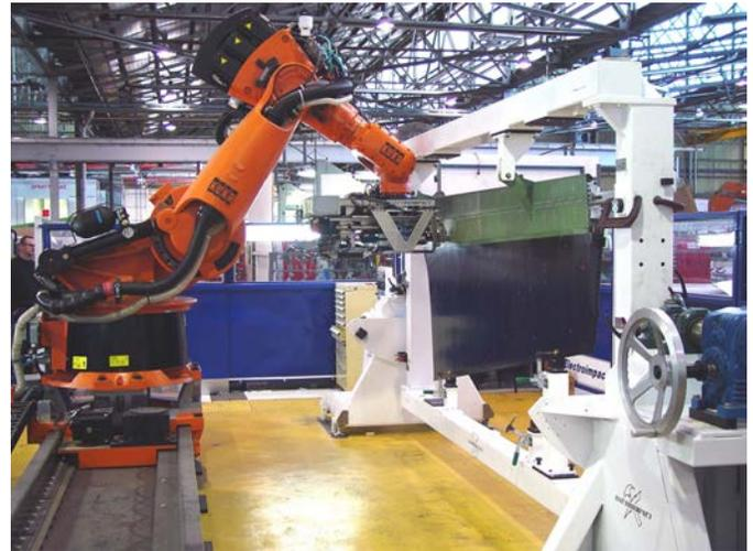
tools that can be configured for a variety of process functions. The end effector has evolved from years of aircraft production and development experience. The robot/MFEE system will drill, countersink and inspect the outer mold line holes of the targeted assemblies. The unique NC programming development, as well as cutter design and process validation, was led by Phantom Works, Boeing St. Louis.
