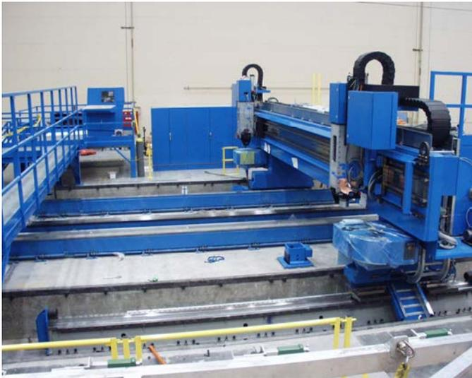
**Figure 1: Gantry Drill Machine
