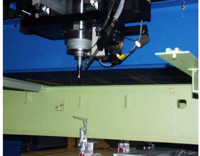
**Figure 7: Coolant Application on Tool**
