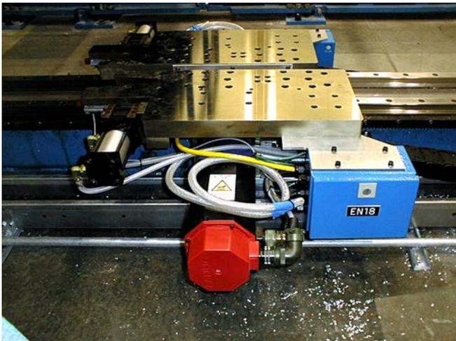
**Figure 4: Material Handling Carriages**
