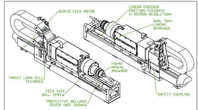
Figure 4: Model 14 Spindle
