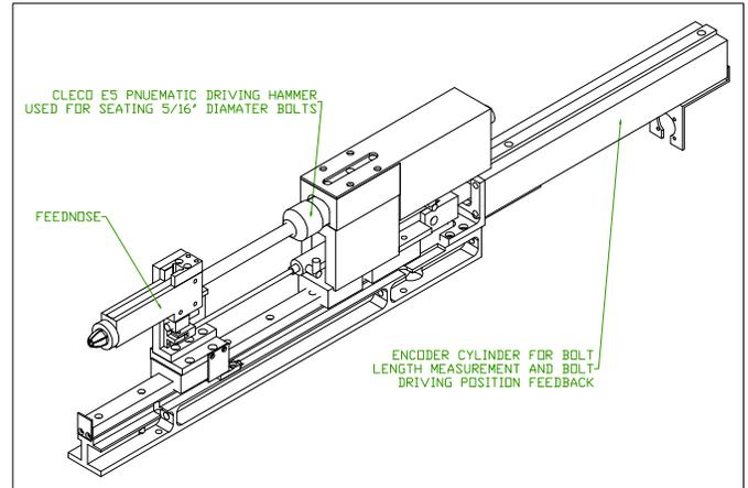
Figure 7: Bolt Inserter
