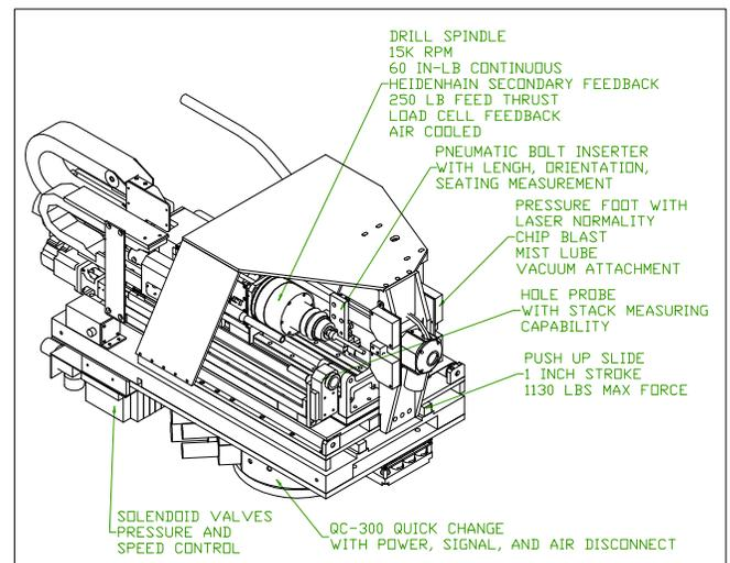
Figure 1: Drill and Drive End Effector
