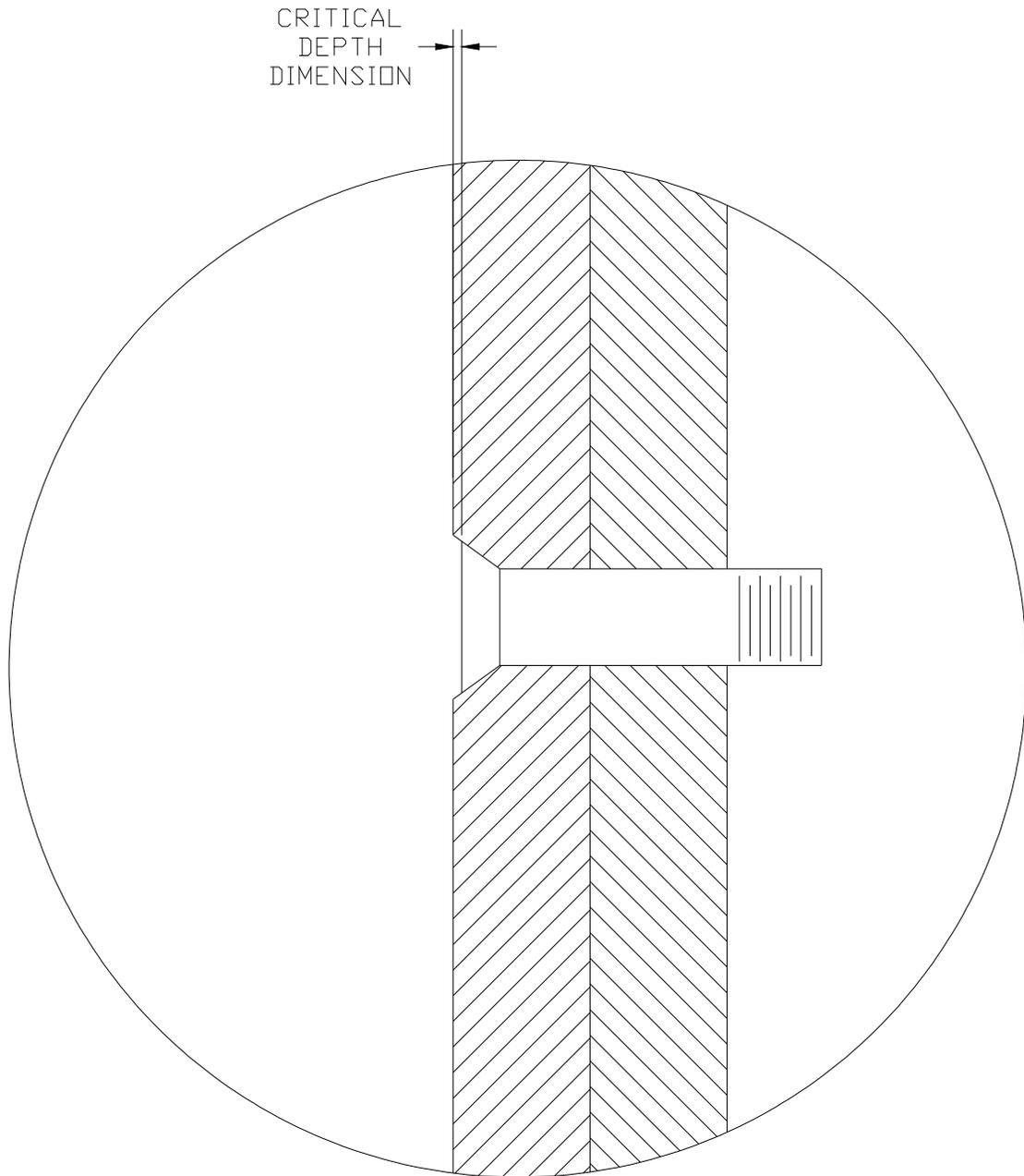
FIGURE 4 – TYPICAL INSTALLED BOLT
