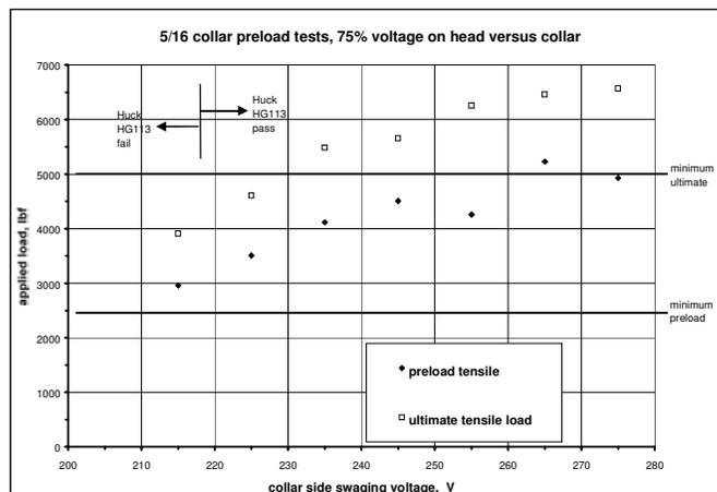
Figure 7. 5/16 Collar Pre-load Tests
