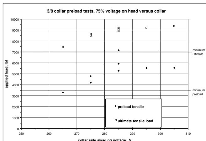
Figure 8. 3/8 Collar Pre-load Tests
