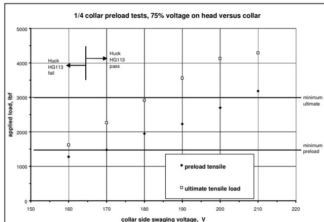
Figure 6. 1/4 Collar Pre-load Tests
