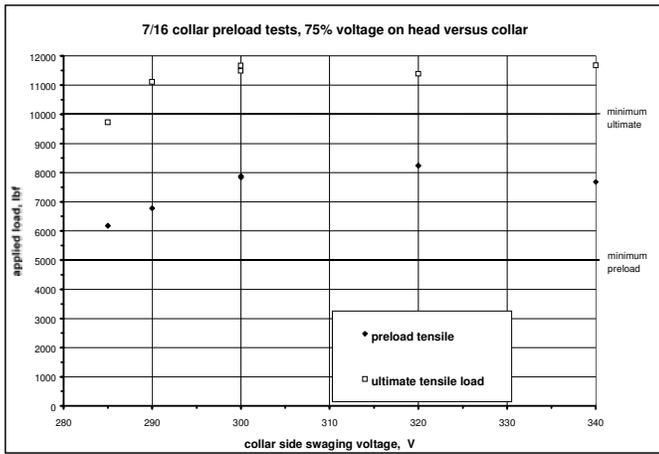
Figure 9. 7/16 Collar Pre-load Tests
