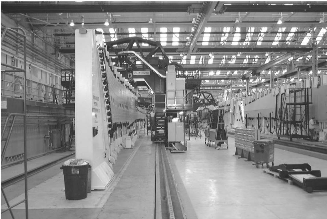
**Figure 6: A340-600 Lower Panel Line: Fill Pass with E4100 Assembly machine**
