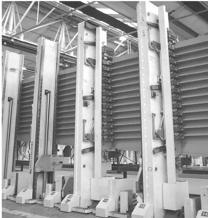
**Fixtute 10: Popping Post Assemblies: Deployed and Stored**
