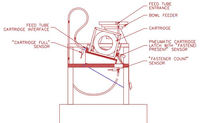
Figure 6. Filling Station Layout
