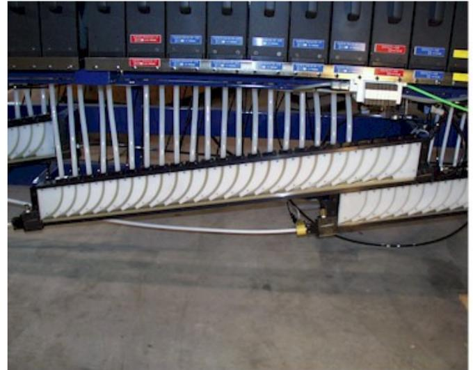
Figure 4. Fastener feed collectors
