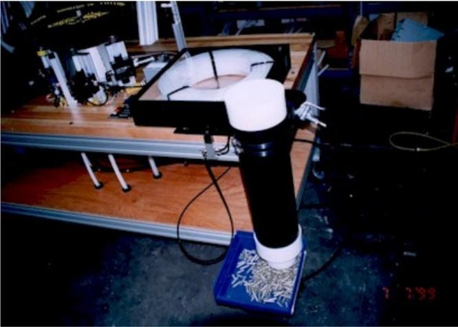
Figure 7. Manual cartridge purge station
