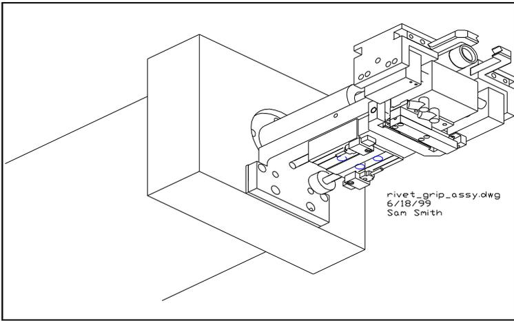
Figure 3: rivet gripper assembled
