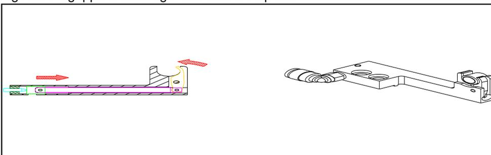
Figure 15: gripper fingers gripping collar
