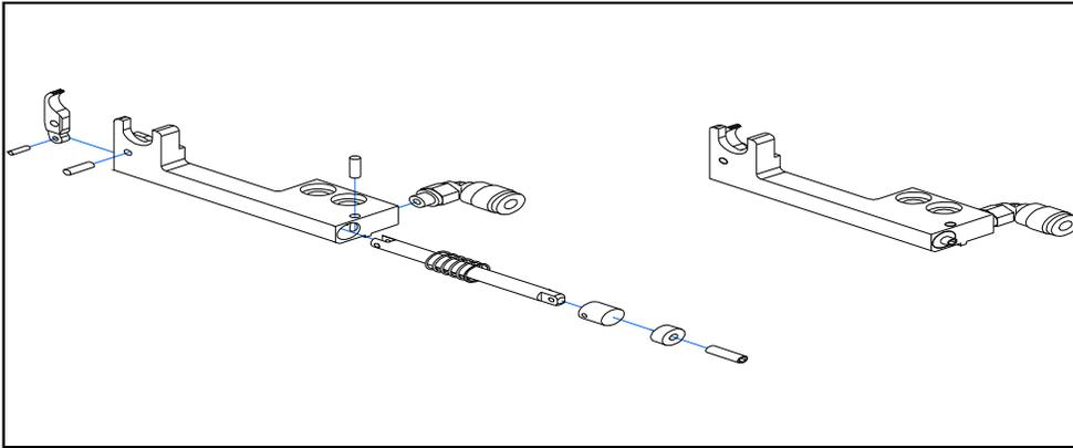
Figure 12: collar gripper (exploded)
