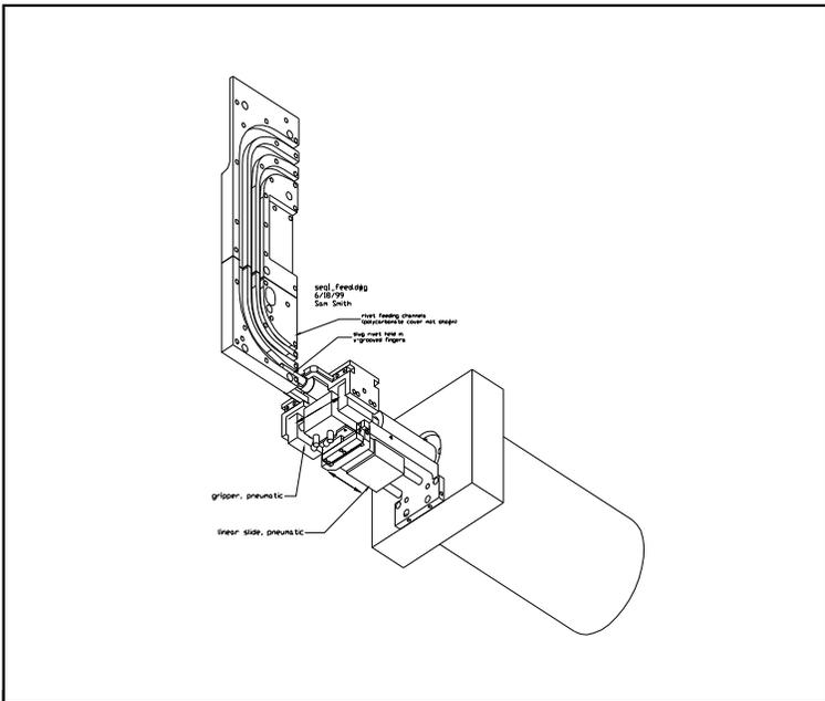
Figure 4: Sequence of operation for the rivet gripper #1
