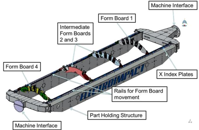
Figure 3: Picture Frame Components
