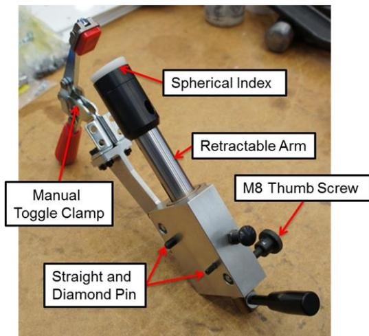
Figure 10: Intermediate Panel Edge Clamp
