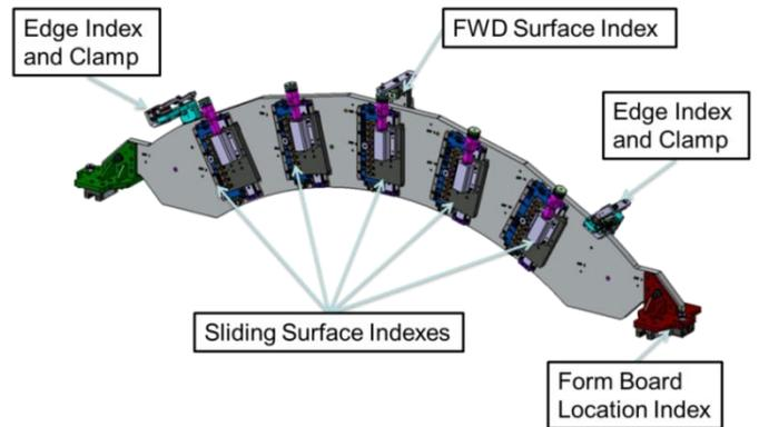
Figure 4: Form Board Components
