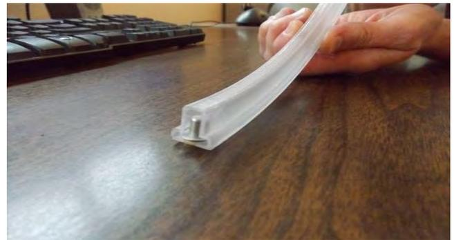
Figure 6 Rivet is blown down a shaped tube to prevent tumbling
