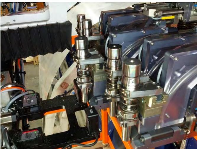
*Figure 11. Injector-mounted automatic anvil tool changer*
