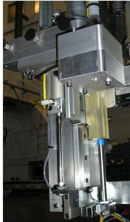
Figure 2 push bolt injector
