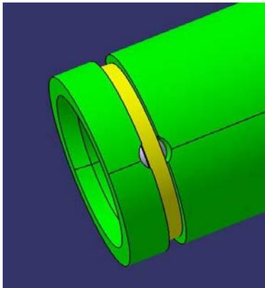
Figure 6: Socket Detent
