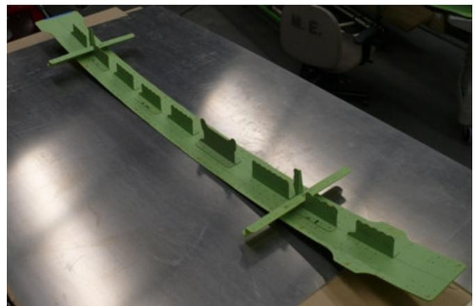
Figure 2. Subassembly of splice plate, shear ties & stringer splices
