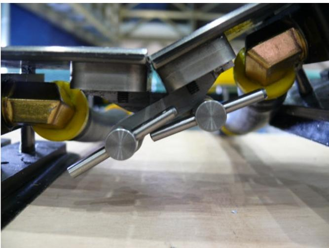
Figure 6. Quick Change Track Splice
