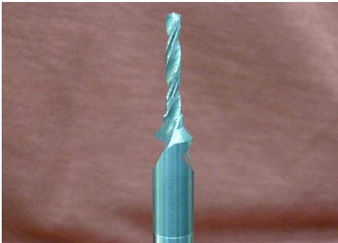
Figure 3. Carbide Drill & Countersink
