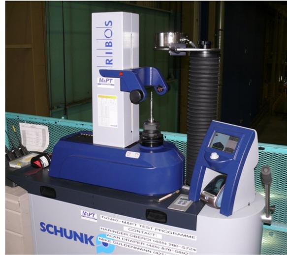
Figure 4. Tool Presetter
