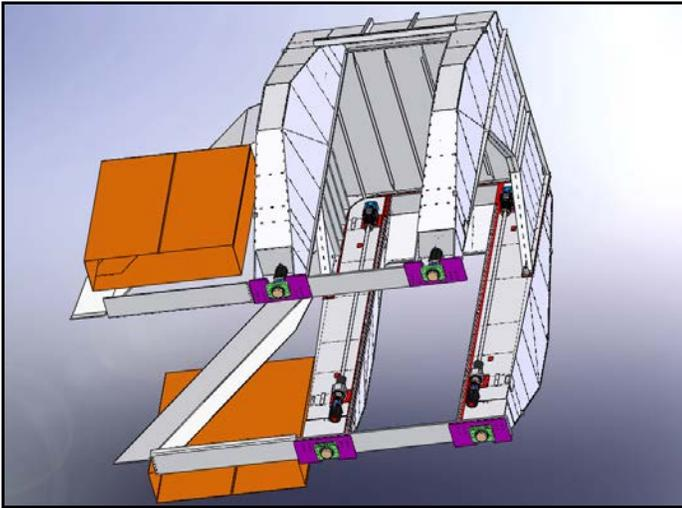
Figure 6. Rigid gantry structure.
