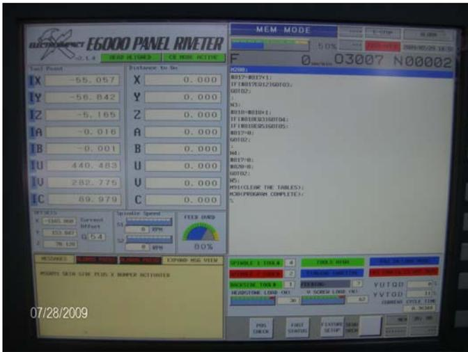
Figure 16: CNC display in Memory mode.
