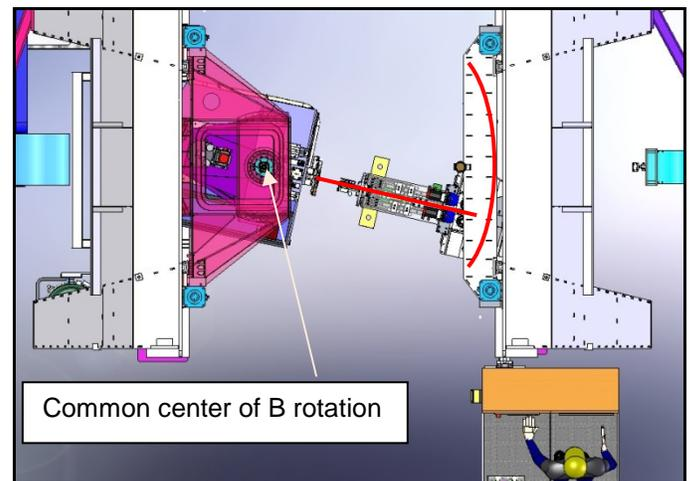
Figure 5. Coordinated head motion at B = -12°.
