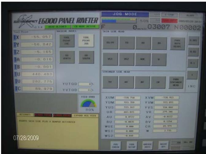
Figure 17: CNC display in Jog mode.
