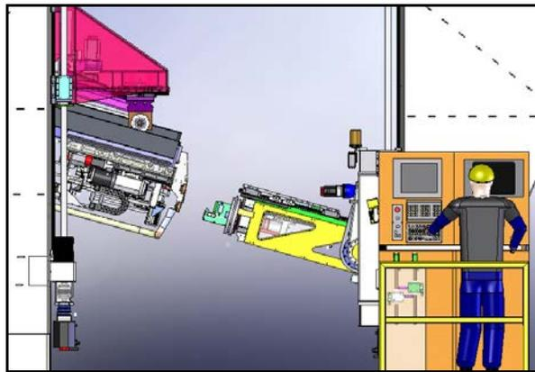
Figure 2. Coordinated head motion at A = -15°.
