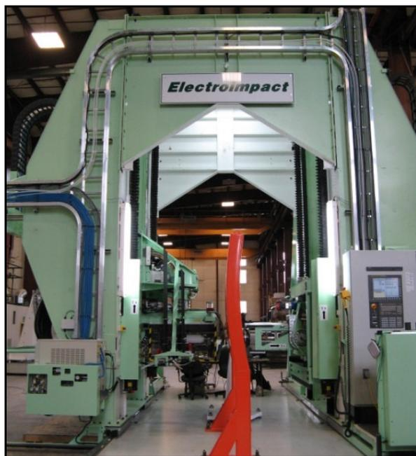
Figure 1. E6000 riveting machine.
