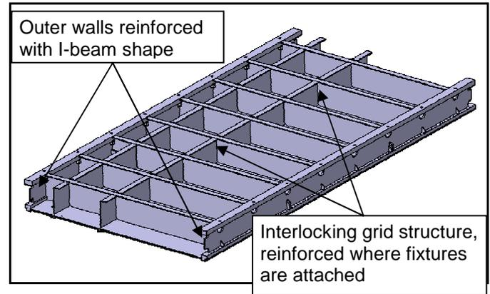
Figure 10. Underside of monolithic bed.
