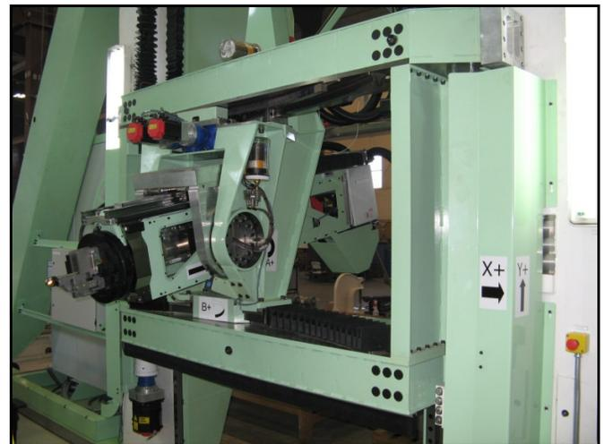
Figure 8. Stringer side Y-A-B-V assembly.
