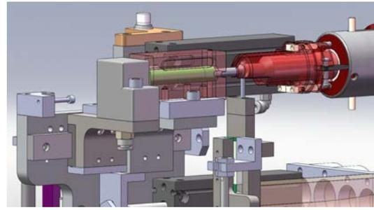
Figure 10 - Bolt injected into bolt inserter fingers
