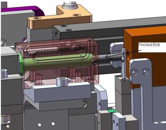
Figure 9 - Chamber extended with a pinched bolt
