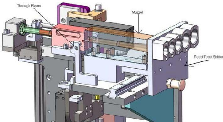
**Figure 4 - Muzzle, Through beam and Feed tube shifter**
