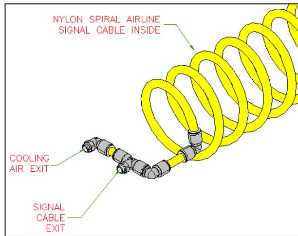
**Figure 4 – Air-Signal Segment (Actuator end)**
