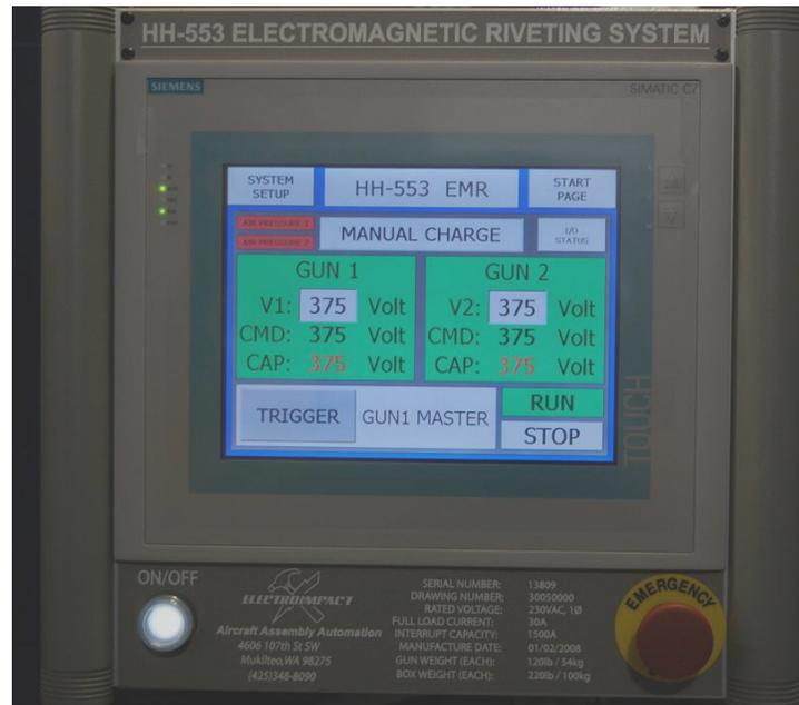
Figure 6 - Siemens Touchscreen PLC
