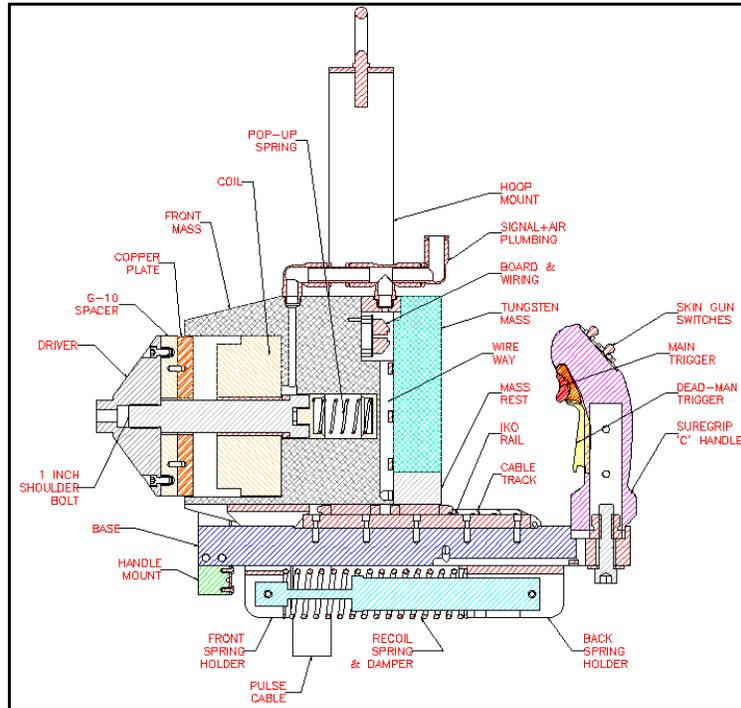
**Figure 2 - HH-553 Actuator Cutaway Diagram**
