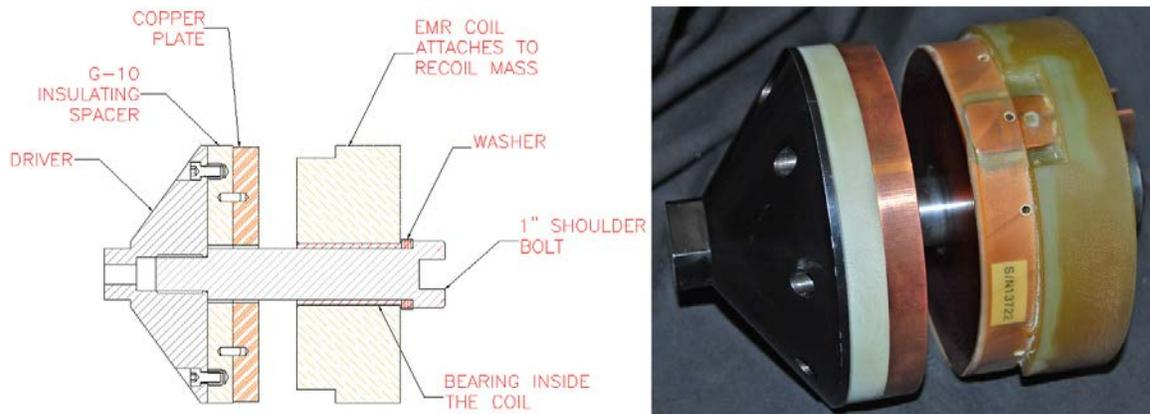
**Figure 3 – Center-less Coil Driver Assembly**
