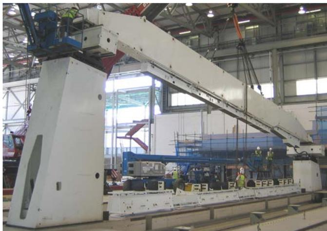
**Figure 1 - Retractable Top Beam Wing Jig**
