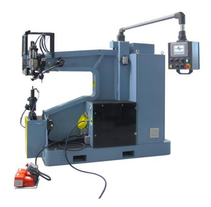
The EI – Portable can be supplied to meet customer's power requirements, and standard shop air of 85 PSI. The EI- Portable utilizes airflow over oil pressure system. In this way, it can be plugged into any standard shop air outlet and a 110 VAC power outlet, or any power requirement specified by the customer.
